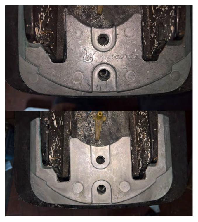
The genuine part SAMPLE "B" (year 2016) was installed with no problem since the holes are perfectly aligned.
